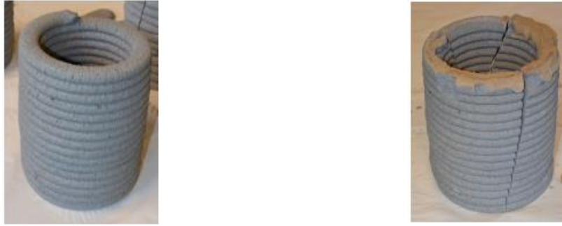
Fig 3. Column printed out of B840/SF/FA/LP: a) before test; b) after compressive strength test [19]
